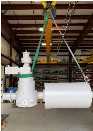
Figure 1 - Example of a Proper Lifting Method, RS
