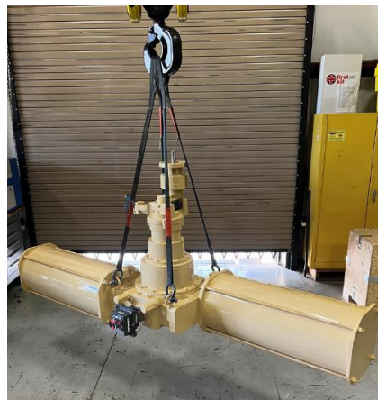
Figure 2 - Example of a Proper Lifting Method, RSDR
